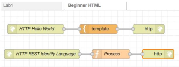
2. Delete the connections between the last three nodes by clicking the connectors and pressing Delete on your keyboard.
