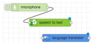
8. Select the **language translator** node. Go to the **info tab** and note that the input is expected on `msg.payload` and the output is on `msg.translation`. The **speech to text** node sends output to `msg.transcription`, but the **language translator** node expects input on `msg.payload`. This means that the nodes cannot be connected directly.
