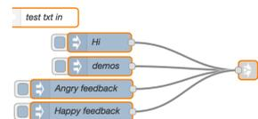
5. Click the **link** node. Note that the text is passed directly to the **tone analyzer** node.
