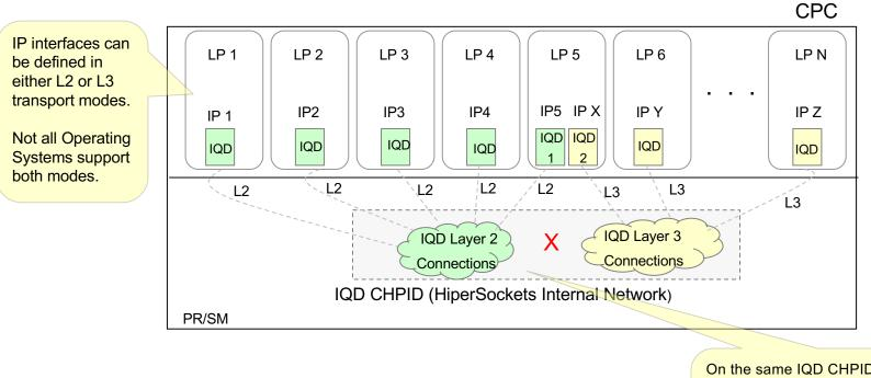
On the same IQD CHPID, the green IQD connections using L2 mode are isolated from the yellow connections using L3. L2 and L3 IQD connections **can NOT communicate** over the same IQD CHPID!
