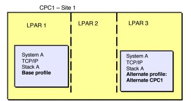
A system image may have multiple alternate locations where it could be running. These could be on the same CEC, same site, or at a different location altogether.
